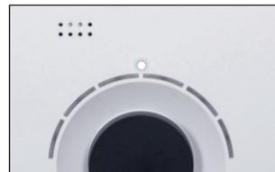
2. To switch off the BONECO appliance while it is in AUTO mode, briefly press the output regulator once.
