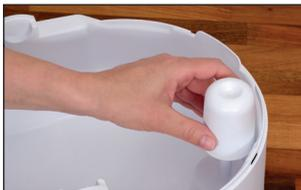
5. Twist both drum discs to release them. When doing so, note the markings on the outer side of the disc.
