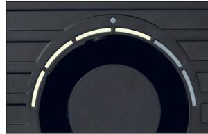
3. Briefly press the output regulator once to exit manual mode and to reactivate AUTO mode.
