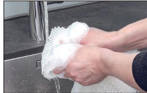
2. Continue to rinse out the AH700 evaporator mat in clean hot water until foam no longer forms.
