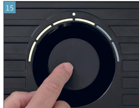
Briefly press the output regulator to switch on the appliance.
