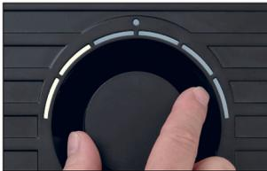
The selected performance level is indicated by the number of LEDs that light up above the output regulator.
