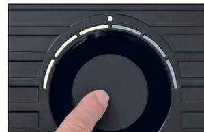
The appliance is always in AUTO mode when it is switched on. You can identify active AUTO mode by the small LED that lights up above the output regulator.
