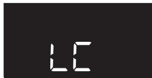
If the output regulator is operated after the LOCK function has been activated through the BONECO app, the LEDs and the display flash 3× in quick succession. If the appliance has been switched off through the BONECO app, the "LC" notice flashes 3× on the display.
