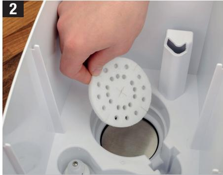
Place the included anti-mineral pad on the heating plate.
