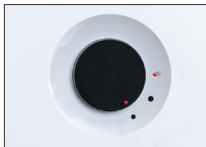
Water tank is empty
